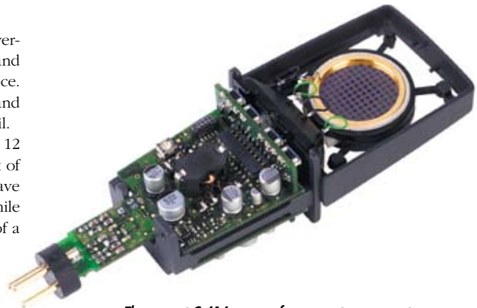
The current C-414 uses surface-mount components, but adds additional polar patterns and filter settings.
